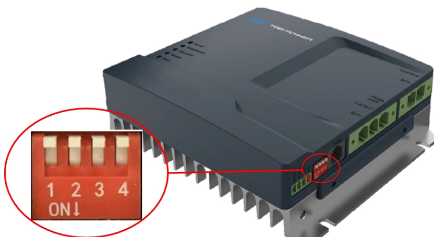
Fig 3- 19 DM series communication address dip setting
