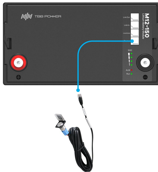
Figure 2-10 Schematic diagram of Battery Switch installation and wiring
