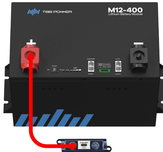
Figure 2-8 Connect the power cable to the lithium battery (+) terminal
