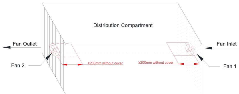
Fig 3-1 Schematic Diagram of Heat Dissipation in Distribution Compartment
